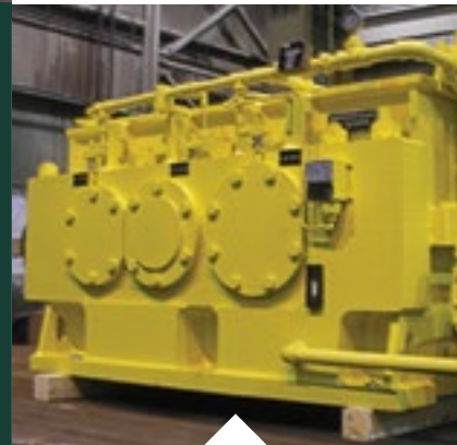
GEARBOX BEFORE Horsburgh & Scott Rebuild & Repair
